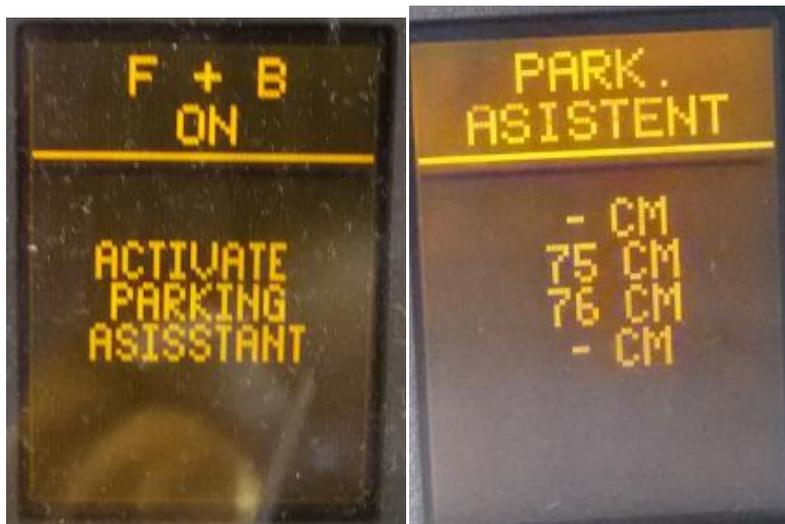
Function will automatically start on reverse gear, if it was activated in the menu and cables is connected. **Function is active only in boardcomputer mode with minimaly one preprogrammed value.**
