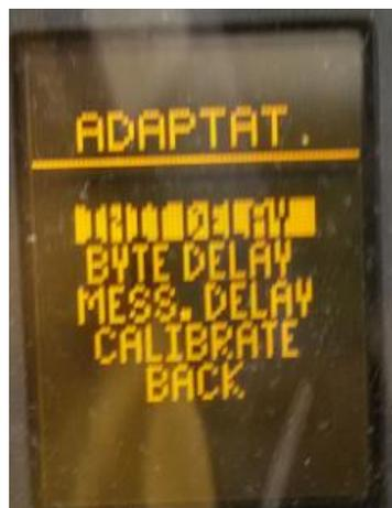
Function "CALIBRATE" will make automatic calibration. It works only on first batch of units (sold before 15.12.2014)
