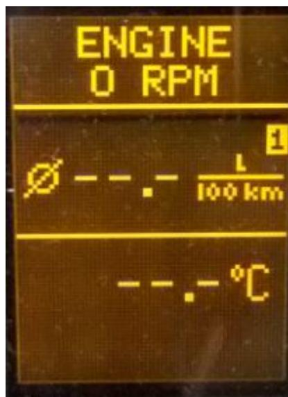
TIP: I strictly recommended to program values from one ECU consecutively. For example values 1,2,3,4,5 from engine ECU and 6,7,8 from Instrument cluster. Not at random, because Maxi-K must always start new communication sequence when the value is from other ECU and it may take several seconds.
